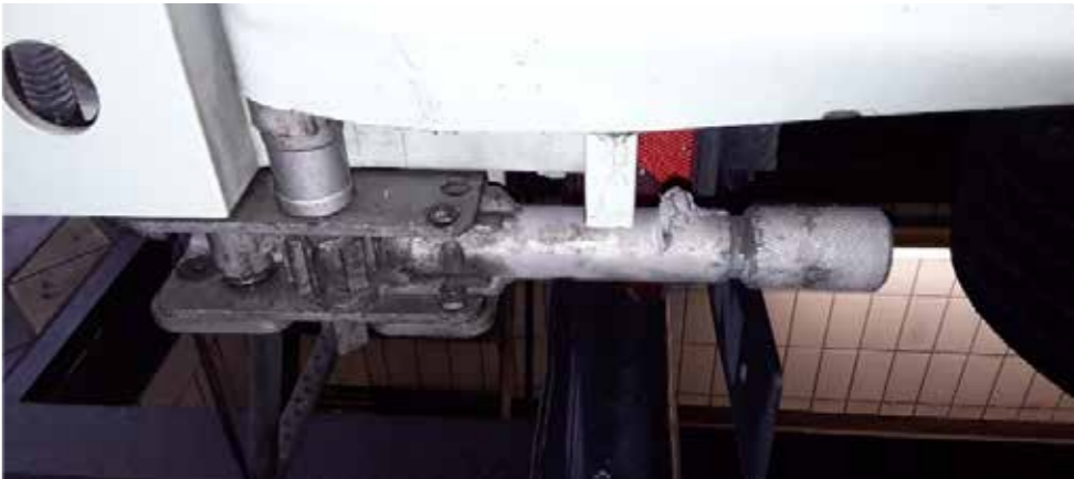
✗ Faulty tarpaulin tensioner
