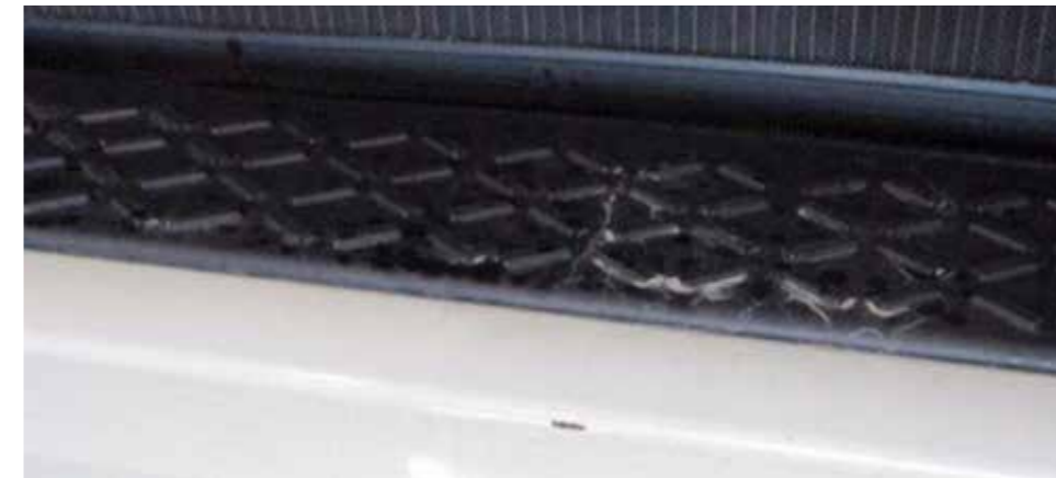
✓ Mileage-related stone damage
