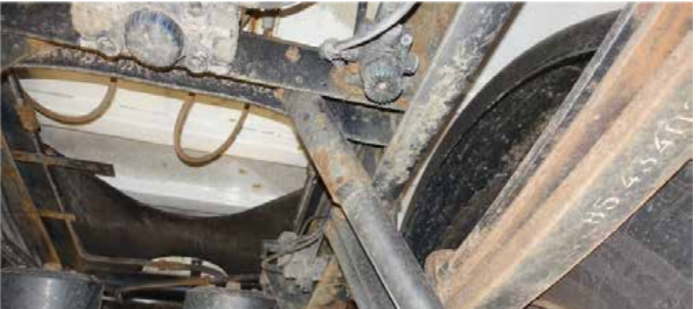
✓ Minor signs of corrosion on the tipper
