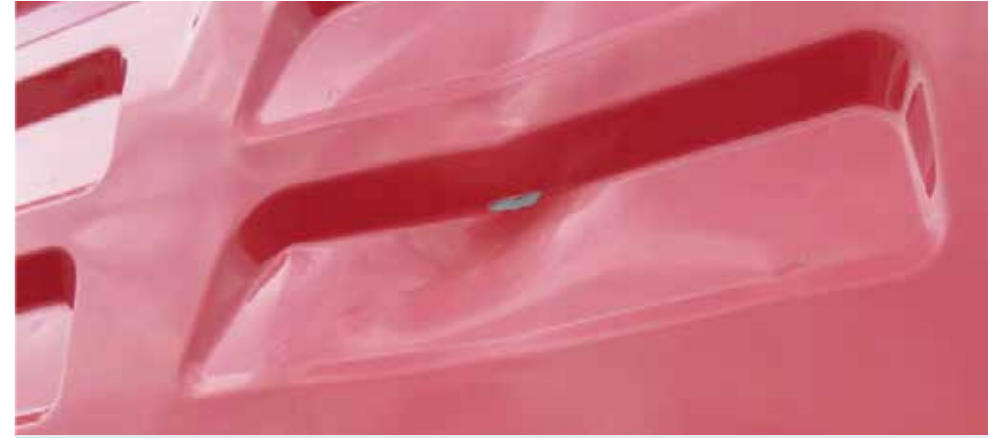
✗ Dented back of cab
