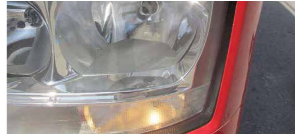
✓ Smaller stone damage, with no formation of cracks
