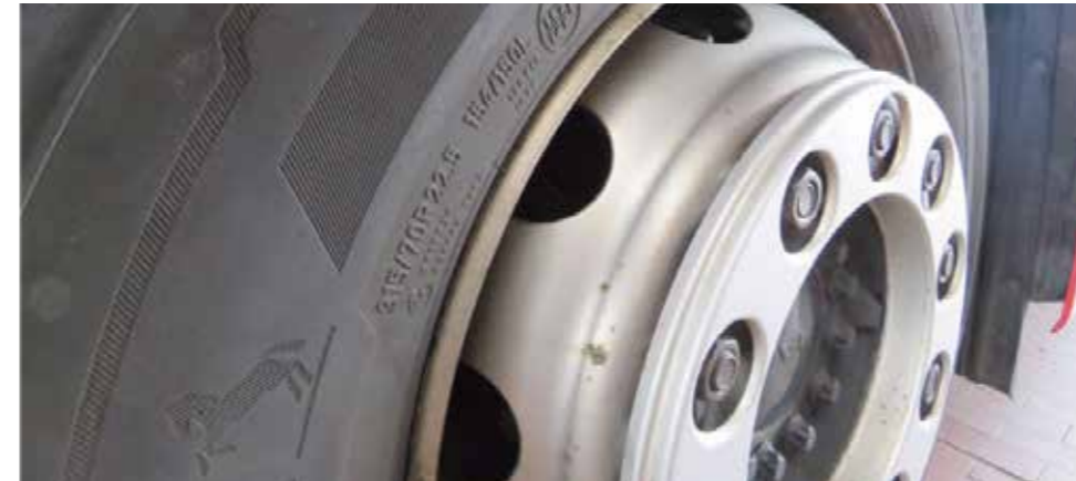
✓ Minor signs of corrosion
