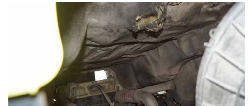
✗ Damaged soundproof matting
