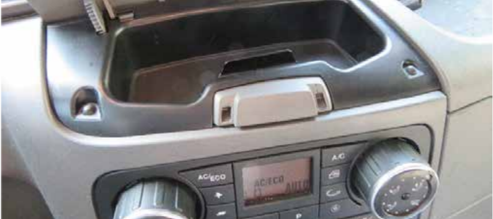
✗ Broken stowage compartment lid
