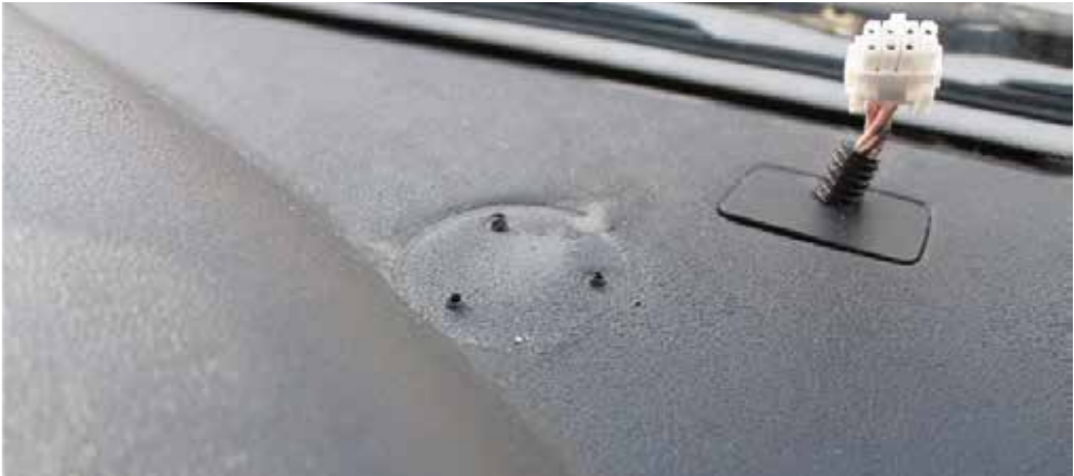
✗ Drill holes in the instrument panel
