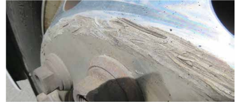
✗ Material abrasion on the wheel
