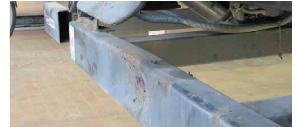
✗ Deformation of underride protection
