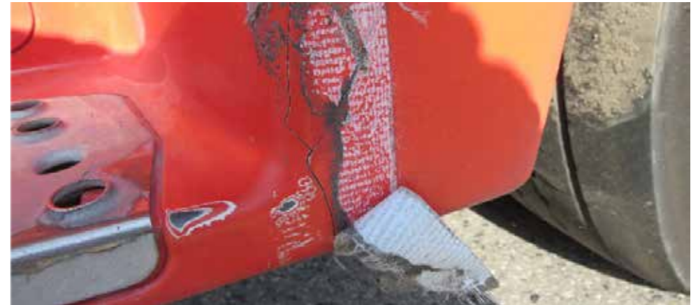
✗ Broken step unit
