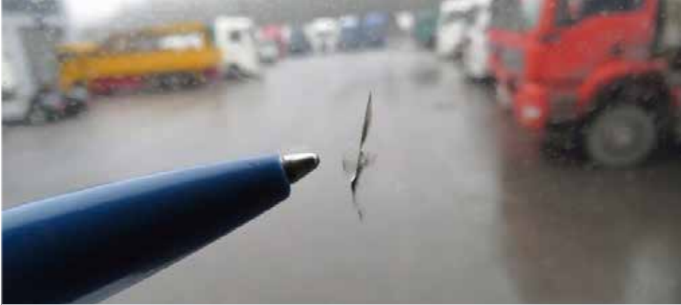
✗ Stone damage with formation of cracks in the field of vision
