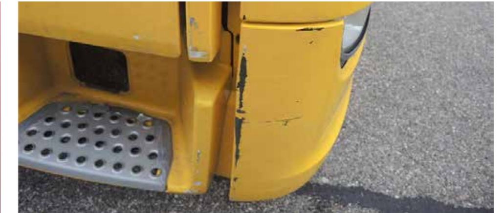
✗ Damage to paintwork
