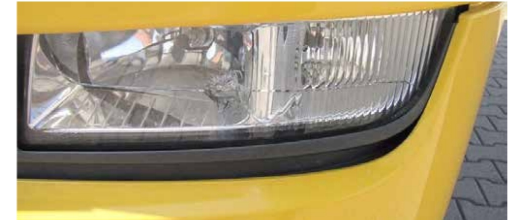
✗ Stone damage with formation of cracks
