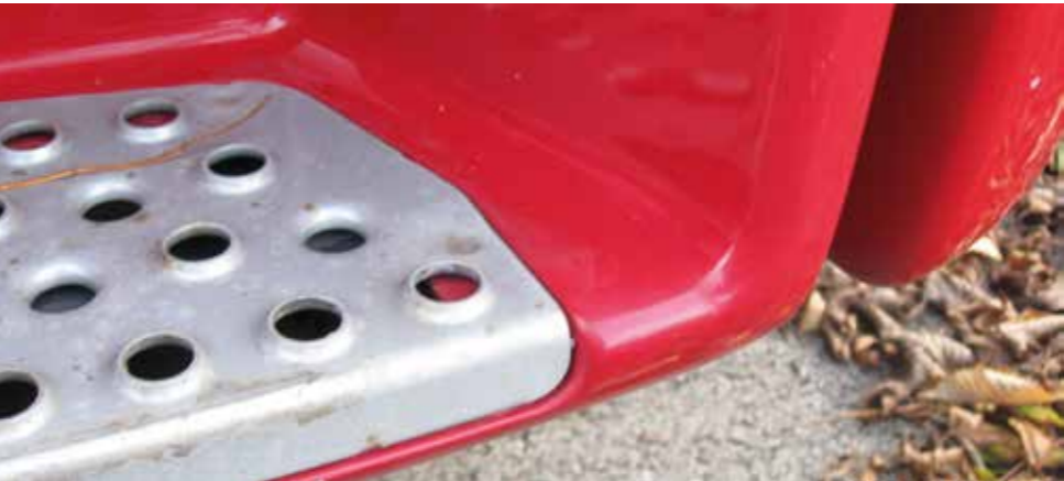
✓ Minor scratches on the step unit
