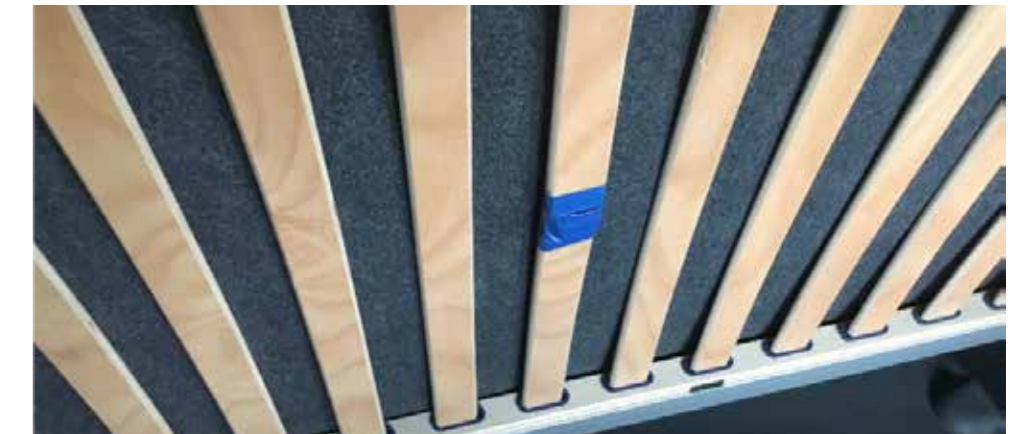
✗ Broken slatted frame
