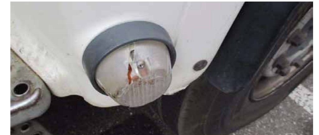
✗ Broken indicator light
